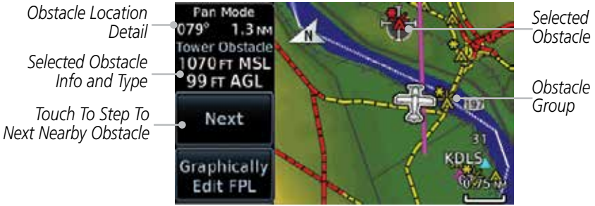
Figure 8-22 Point Obstacle Detail
