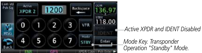
Figure 2-7 Transponder Mode "Standby" Indication
