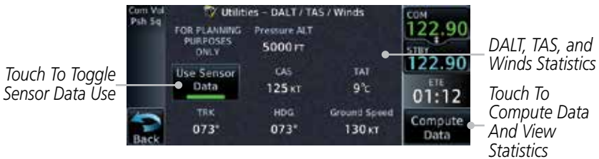
Figure 14-37 Utility DALT/TAS/Winds Page Using Sensor Data and Pressure Altitude
