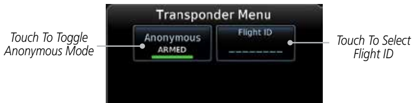
Figure 2-14 ADS-B/Transponder Control Panel
