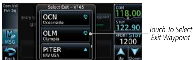
Figure 4-21 Select an Exit Waypoint for the Airway
