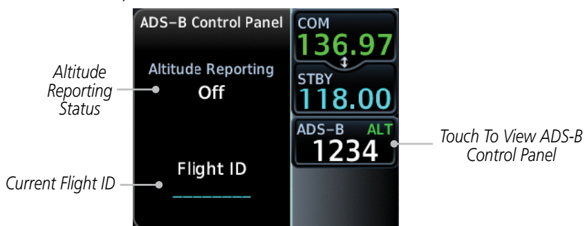
Figure 2-13 ADS-B Control Panel
